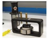
Install the special assembly lower into the maintenance fixture, which can be either bench or vice mounted.
