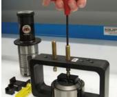
Use the T-handle wrench (supplied) to compress the springs in the lower assembly to allow access to the retaining ring.
