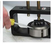
Use the screwdriver (supplied) to remove the retaining ring(s) from the lower assembly, releasing the stripper plate.
